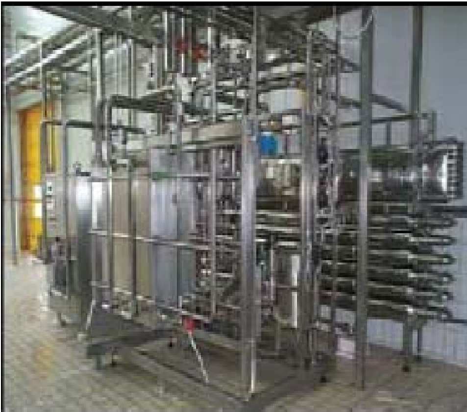
Pasteurizer with tubular heat exchanger and plate heat exchanger
